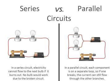
In a Series Circuit, resistors are connected end-to-end so that the current flows sequentially through each resistor. The series circuit's total resistance is equal to the sum of the resistors' individual resistances. This means that the total resistance of the circuit increases as more resistors are added in series.
